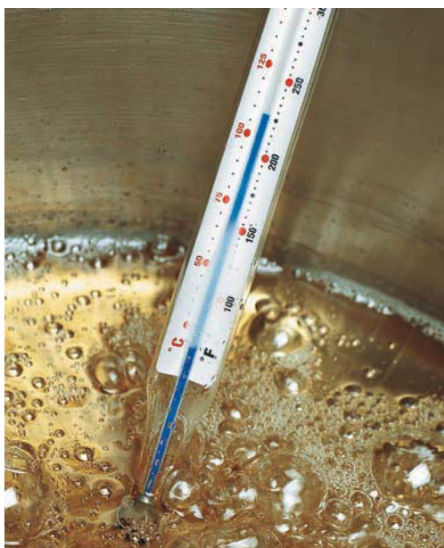
Sugar dissolved in water to make candy causes the boiling point to be elevated above 100°C.
